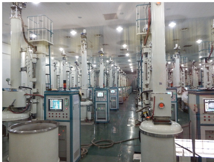
Ingot Growing process No 1 Dept. 100units, (total has 5 Depts , totally 480-units now.)
