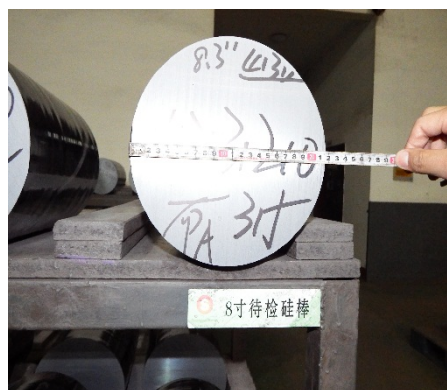
Top and tails cut : No 1 Dept. mainly diameter is: 8 to 8.3 inch . this Dept can cut 250 ingots/day.
