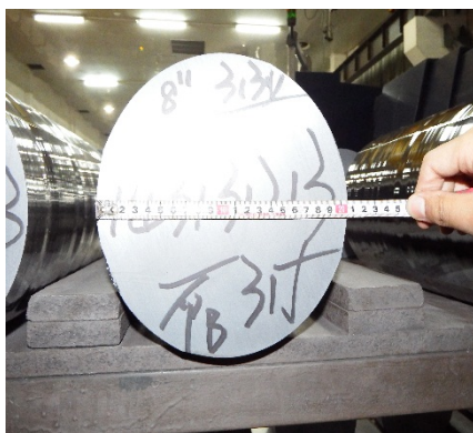
Top and tails cut : No 1 Dept. mainly diameter is: 8 to 8.3 inch . this Dept can cut 250 ingots/day.
