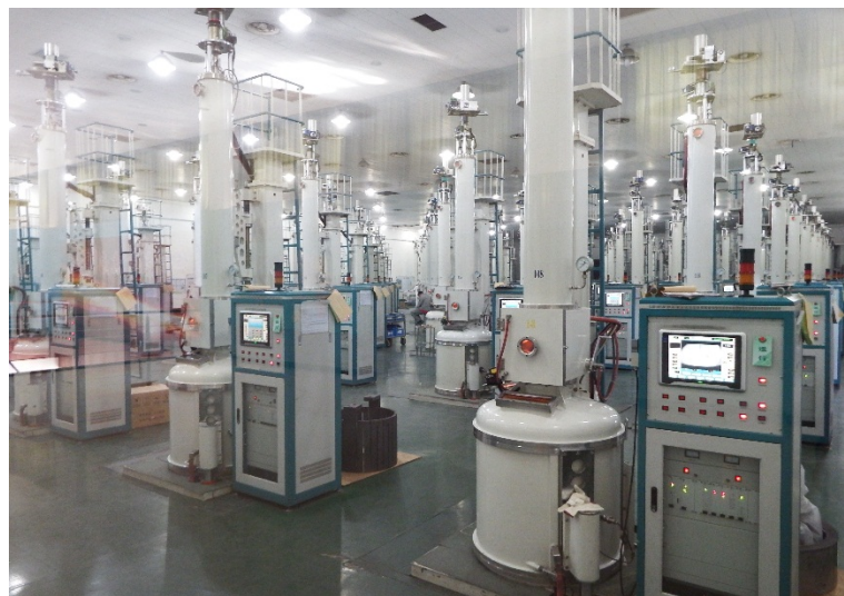
Ingot Growing process No 1 Dept. 100units, (total has 5 Depts , totally 480-units now.)
