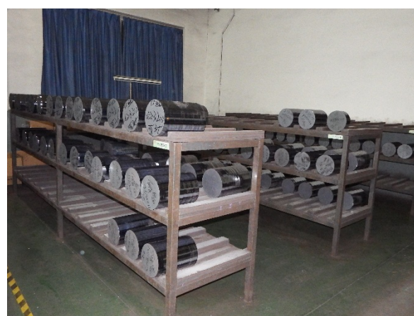
Top and tails cut : No 1 Dept. mainly diameter is: 8 to 8.3 inch . this Dept can cut 250 ingots/day.
